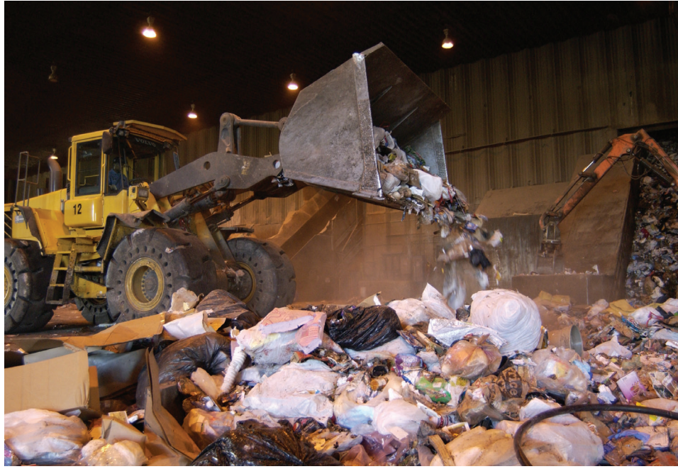
At the Elk River Resource Processing Plant municipal solid waste is processed to create a refuse-derived fuel which is used to generate renewable electricity.
